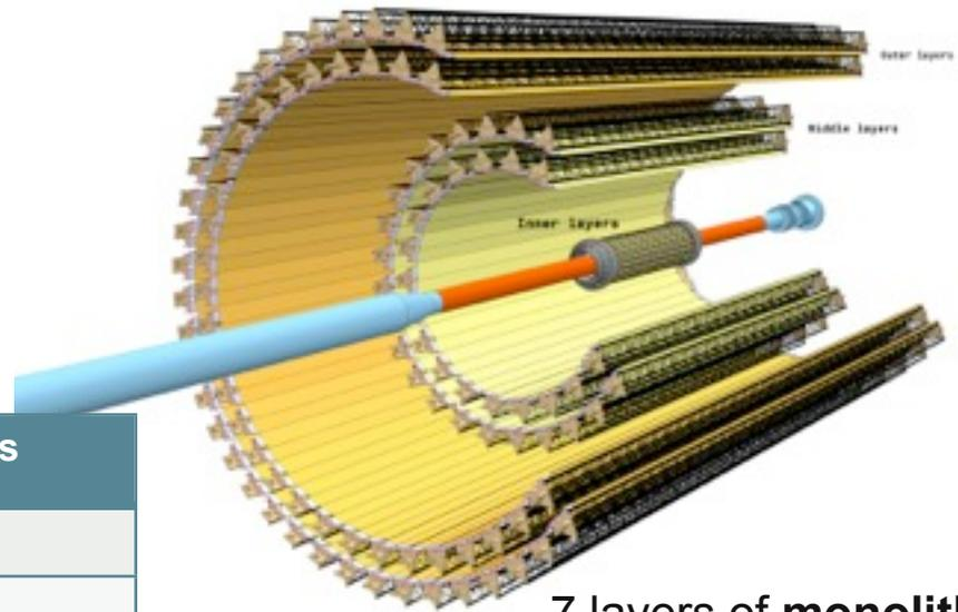
7 layers of **monolithic pixel detectors**
