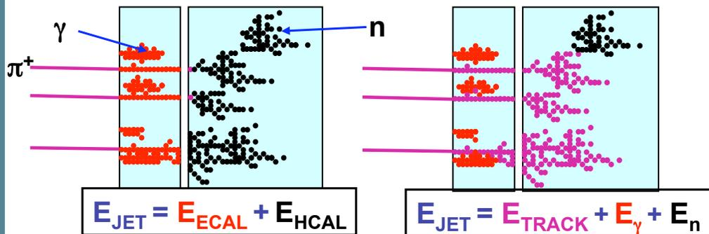
Particle flow = granularity
