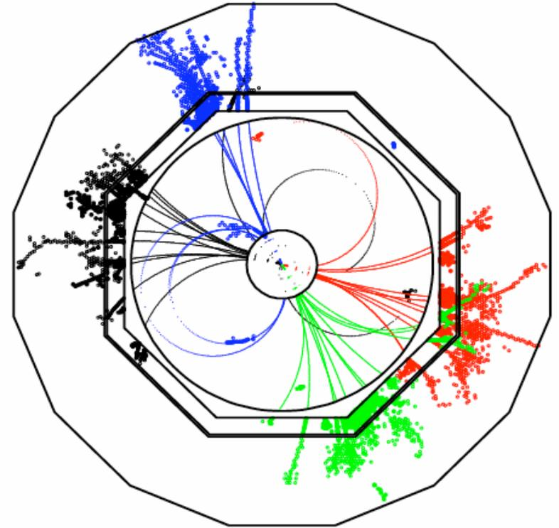
Extensively developed & studied for Linear Collider Detectors: Jet energy resolution goals (3% - 4% or better for energies from 45 GeV to 500 GeV) can be met
