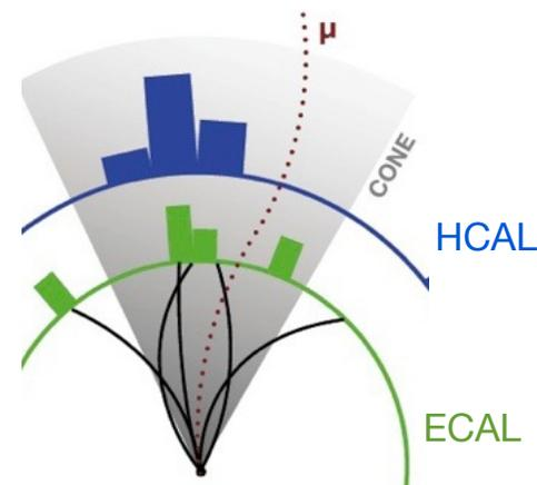
The principle of jet reconstruction: Sum energy in a cone (geometry etc given by jet finding algorithm) to determine energy of original parton
